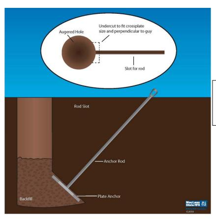
This is a typical installation. Care should be taken not to damage the rod's protective coating when tamping down the backfill.
