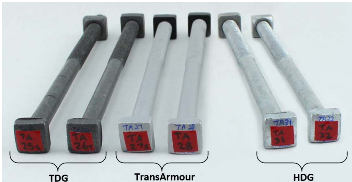
Figure 8: Bolts before cyclic UV/Salt Fog (preconditioned with sand abrasion)
