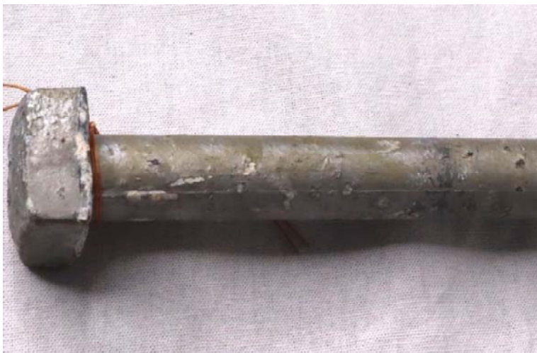
Figure 20: TransArmour-coated bolt, gravel impacted/after cyclic corrosion exposure; zoom in view, no undercutting observed
