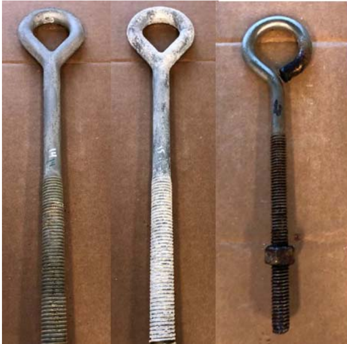
Figure 16: Test items at the end of cycle 5 (Left to right: TransArmour, hot dip galvanized, Stainless steel)
