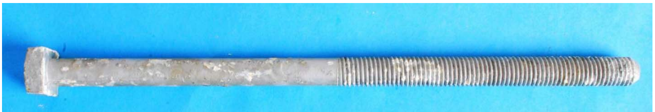
Figure 19: TransArmour-coated bolt, gravel impacted, after cyclic corrosion exposure
