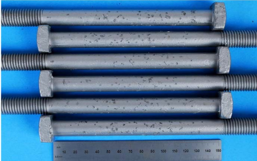
Figure 18: TransArmour-coated bolts after gravel impact (before cyclic corrosion testing)
