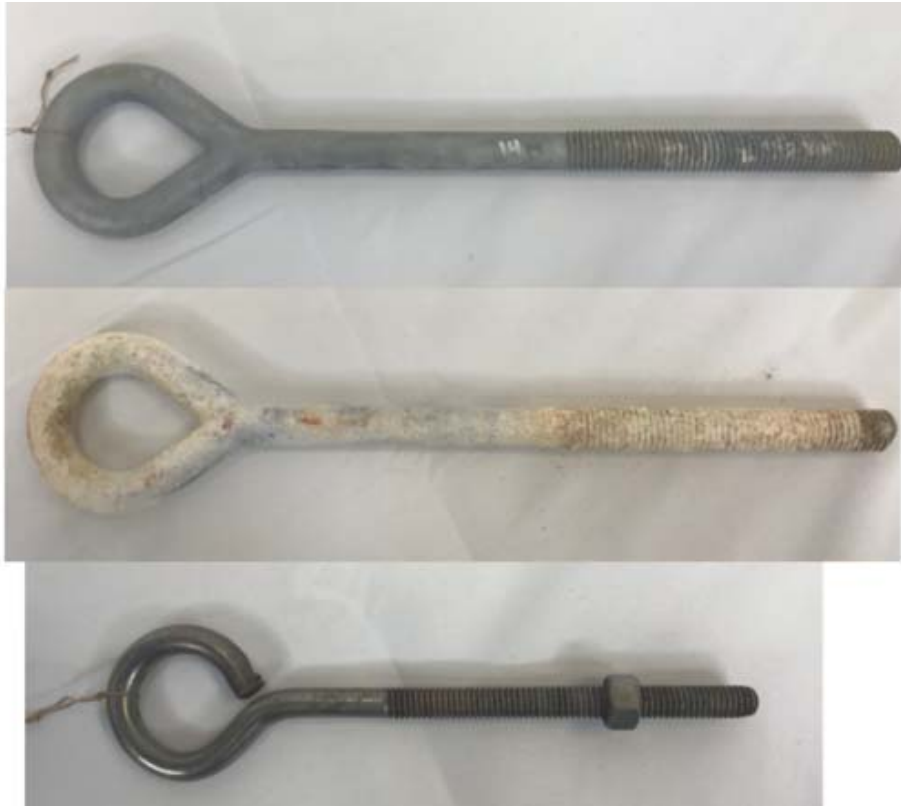
Figure 17: Test items at end of cycle 10 (top to bottom: TransArmour, Hot Dip Galv, Stainless steel)
