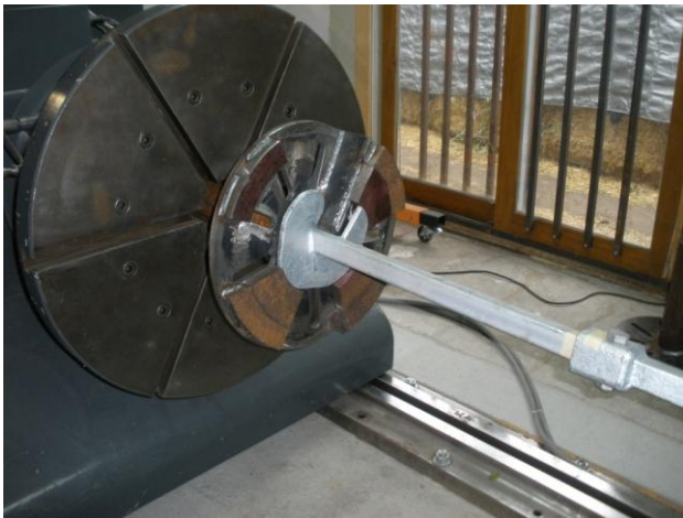
Torque testing with lead and extension in the laboratory
