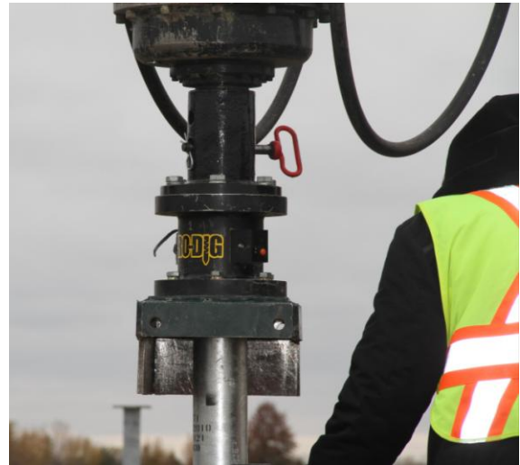
Load cell type torque measuring device.
