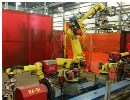
Robotic welding for consistent quality
