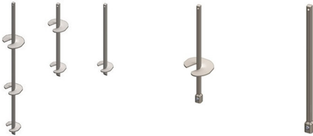
1-1/4 Inch Round Shaft Leads; 7 foot length 2,300 ft-lb Ultimate Installing Torque 23,000 lb Ultimate Tension Load
